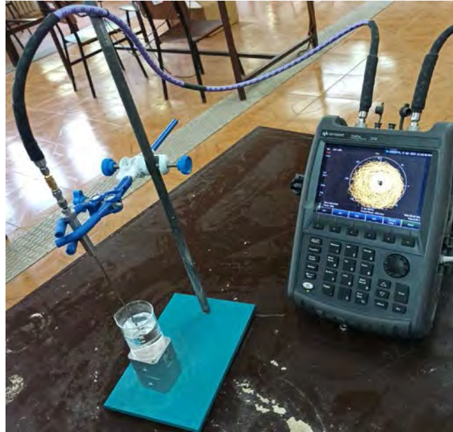
Figure 4. Experimental setup for dielectric constant measurement of oil samples
