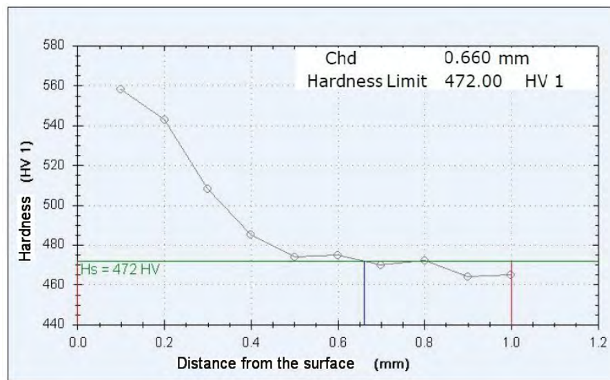
Figure 3. Effective case depth results
