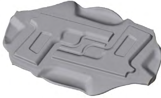
Figure 5: Numerical result of the Hot Forging
