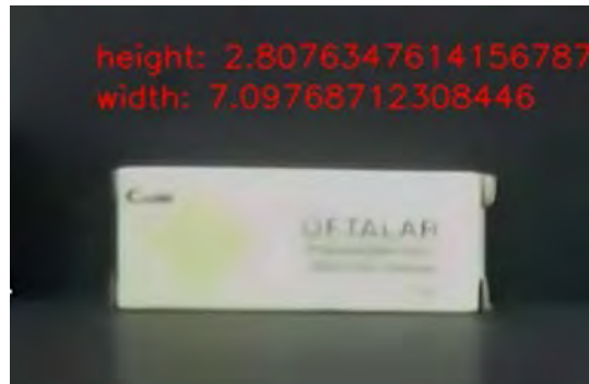
Figure-2: Example of Dimension Measurement with Image Processing
