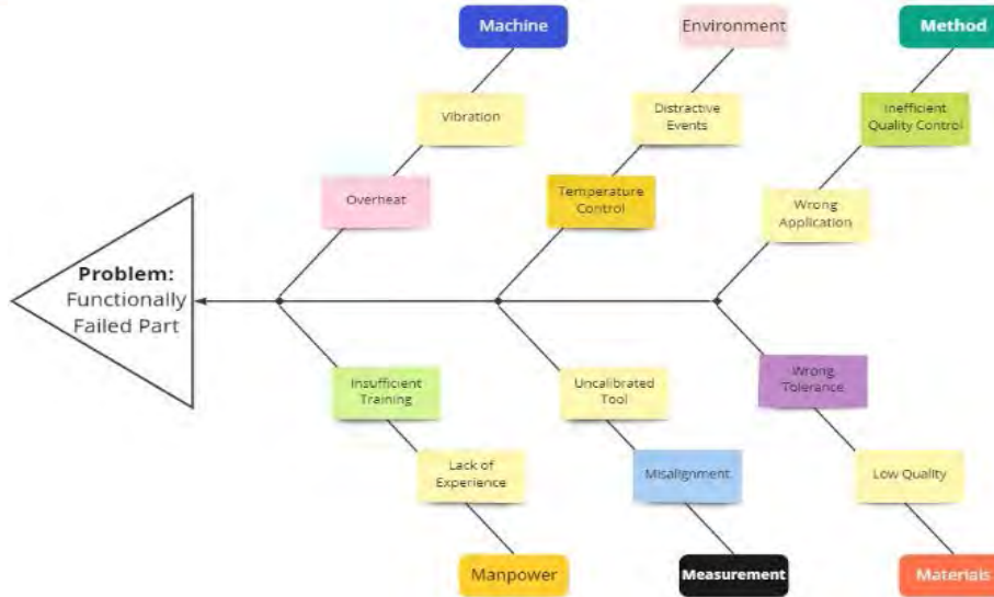
Figure 8: Fishbone diagram for functionally failed part error.
