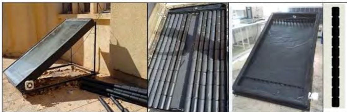
Figure 1. Solar collector equipped with an absorber with can pipes.
